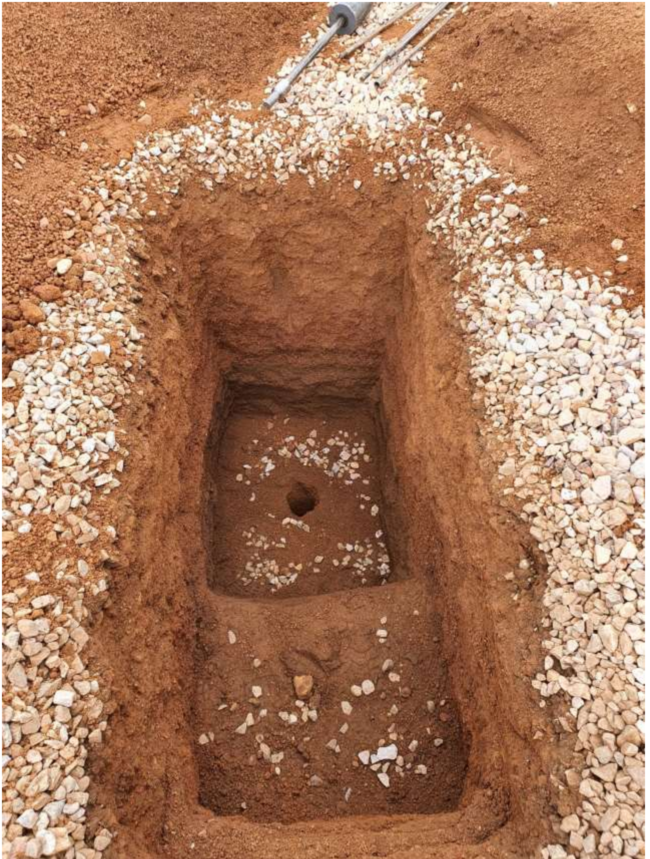
TP1 /AH1_Note gravel ferricrete recovered from TP1
